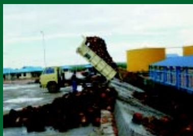
Unloading of FFB at the mill
